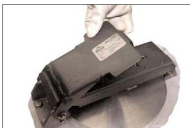
Closing the fill hole cover takes place in reverse order, whereby only the use of the square wrench is no longer necessary.
