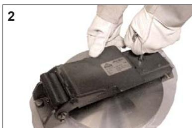
with one hand hold the tension lever and with the other hand turn the square wrench ccw by approx. 90°. The tension lever will be unlocked.
