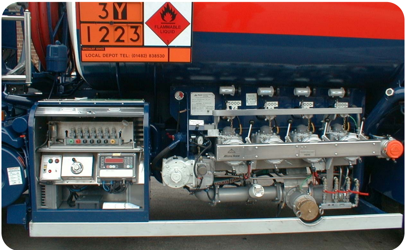
Picture shows typical turbine meter installation with pump
